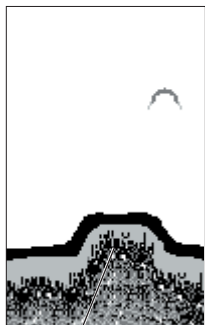
Structure is soft— probably a mud pile
